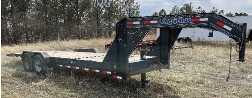
Load Trail 24' tilt-deck w/ 6' deck & 18' tilt bed
